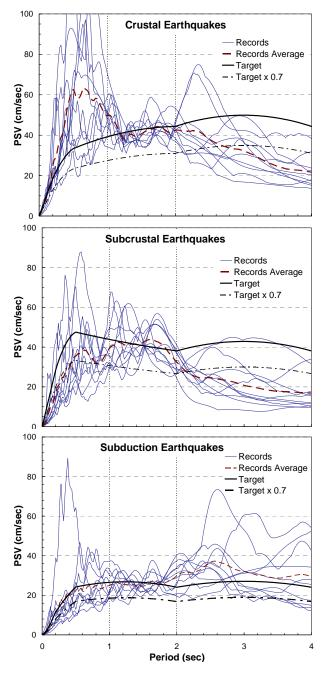
Figure 3. Spectral 5%-damping pseudo-velocities of selected/modified records and target hazard spectra for crustal, subcrustal and subduction earthquakes for the city of Vancouver, BC, in Site Class C (firm ground).
