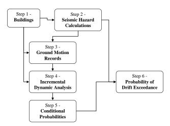
Figure 2. Calculation procedure of risk or the probability of drift exceedance, PDE, for BC school structural systems.
