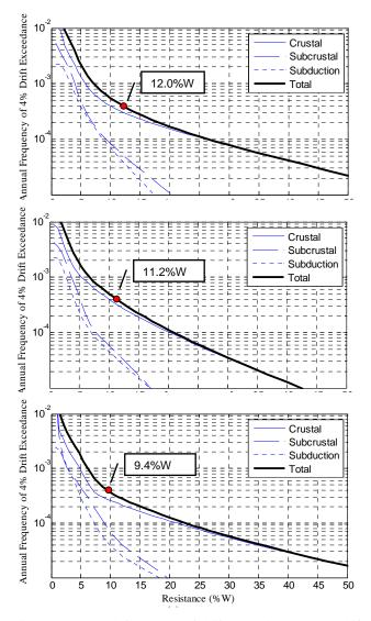
Figure 7. Annual frequency of drift exceedence at 4% drift limit for prototypes S-1, S-7 and S-8 for site class C in Vancouver
