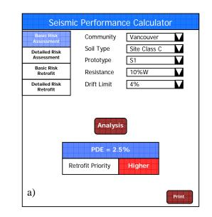
Figure 9. A preliminary version of the Seismic Performance Calculator for the seismic risk assessment/retrofit of BC schools
