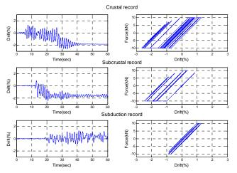
Figure 6. Displacement histories and hysteresis curves of the S-8 model for the crustal (top), subcrustal (middle) and subduction (bottom) records.
