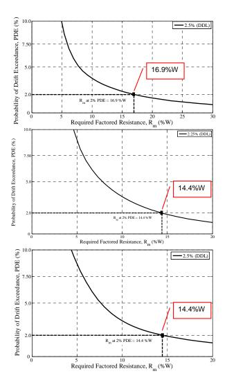
Figure 8. Probability of Drift Exceedance at DDL for prototypes S-1 (DDL=2.5%), S-7 (DDL=2.25%) and S-8 (DDL=2.5%) for site class C in Vancouver
