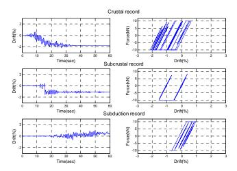
Figure 5. Displacement histories and hysteresis curves of the S-7 model for the crustal (top), subcrustal (middle) and subduction (bottom) records.
