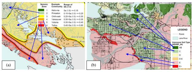
Figure 1 (a) Seismic Hazard Map for South Western British Columbia and (b) Soil Type Map for the Greater Vancouver Regional District
