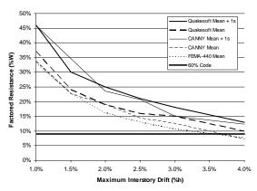
Figure 4 Validation Results for Steel Braced Frames (Tension Only)
