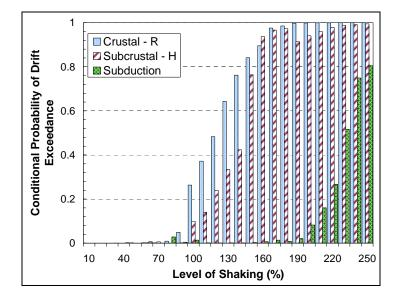
Figure 2. Conditional probabilities of 4% drift exceedance for the three earthquakes for a W-2 located in Vancouver with 10%W resistance
