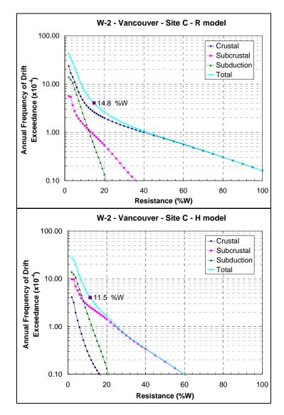
Figure 3. Annual frequencies of 4% drift exceedance of the W-2 prototype located in Vancouver The total annual probability (Eq. 3) is 0.7‰, which is equivalent of having one drift
